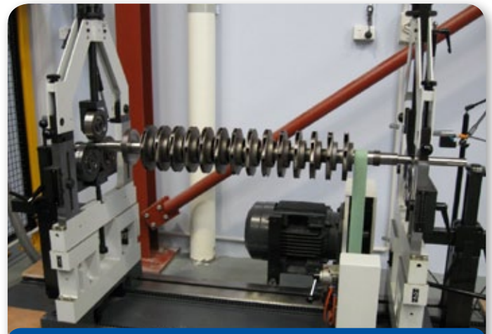
Boiler feed pump rotor dynamic balancing in Perth
