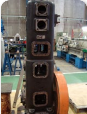
Compressor - after strip down
